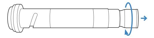
1 Unscrew the optical tip of the probe to remove it
