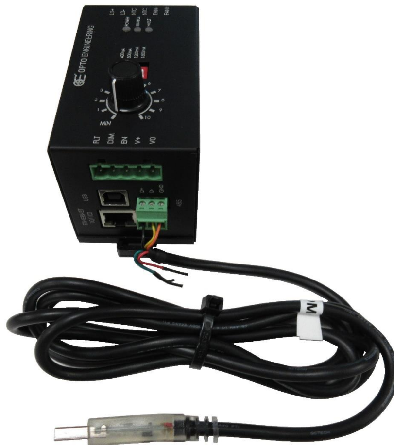
Figure 23: connection of RS485-USB adapter to the controller
