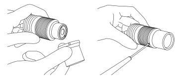
Insert back in place the C-mount adaptor and fix it by tightening the socket head set-screws with an M1.5 Allen key
