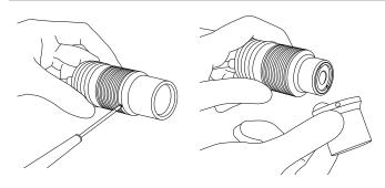
1 Loosen the socket head set-screws by means of an M1.5 or M2 Allen key and remove the C- mount adaptor
