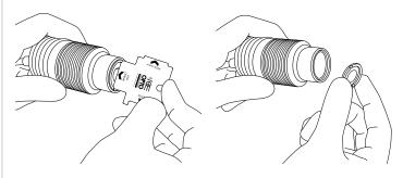
2 Remove the retaining ring using the provided PTTOOL instrument.
