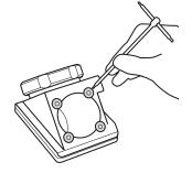
Remove the four holding buttons using an Allen key (M3 screws)
